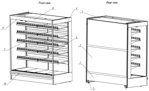
Figure 1 - Main units of the display case
