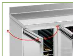
Doors with dual-effect hinges (self-closing at <90^\circ and hold-open at >90^\circ )
