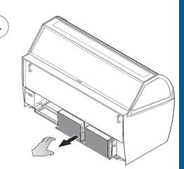
Remove the condensing unit as shown.
