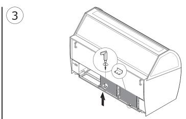
Remove the fixing brackets as indicated.
